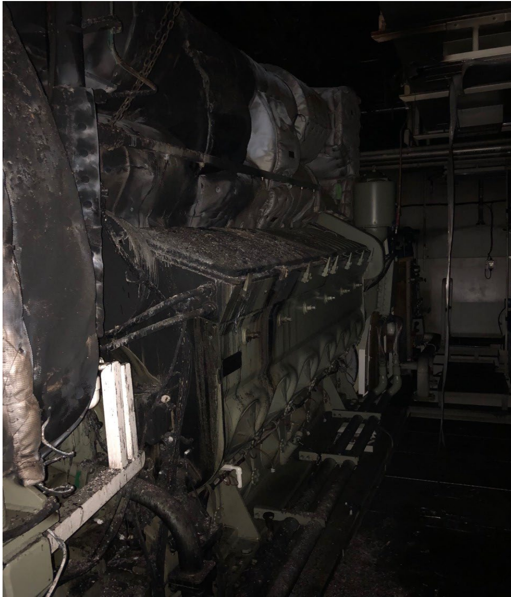
Figure 8. Photograph of the #2 main diesel engine (inboard) post-casualty, facing the New York End of the SANDY GROUND taken on December 23, 2022. Provided by the U.S. Coast Guard.
