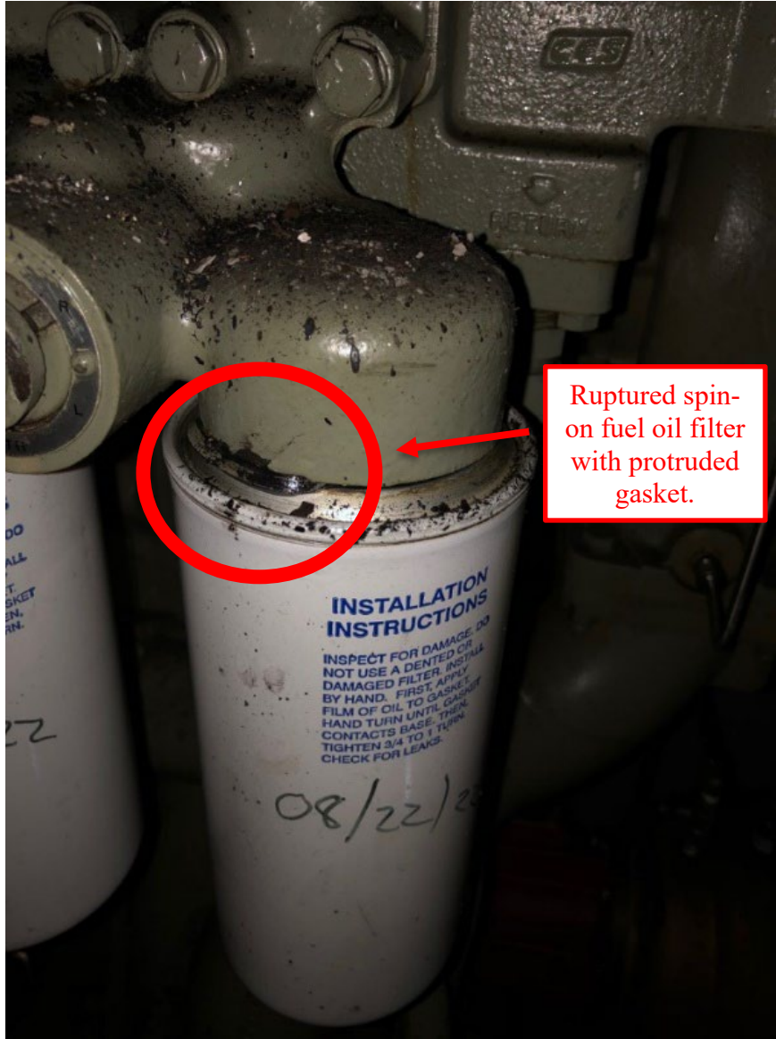
Figure 6. Photograph of the ruptured #1 main diesel engine online spin-on fuel oil filter with protruding gasket taken on December 23, 2022. Provided by the U.S. Coast Guard.
